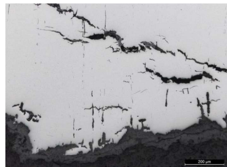
Figure 9. Cantilever F-Top higher magnification image of subsurface secondary cracking near the fracture face.
