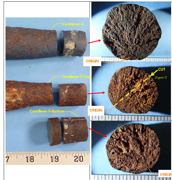
Figure 4. Fracture faces of each PT bar with labeled origin and side lighting. Note the Cantilever A fracture face has blue paint specks across the fracture face.
