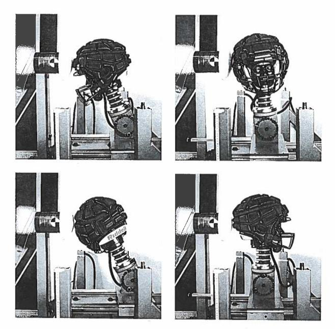
We tested each helmet add-on using our rigid pendulum impactor face, following the same procedure we use in our standard varsity football helmet testing. This yielded 192 impact tests. Additionally, we conducted an extra series of tests where the impactor face was covered with the same add-on as the helmet being tested. This
