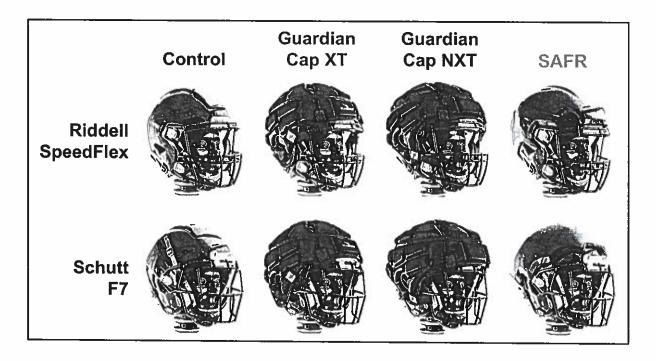
Our <u>varsity football helmet testing protocol</u> includes four impact locations: the front, front boss, side, and back. Each location is tested at three different impact speeds, set at 3.1 m/s, 4.9 m/s, and 6.4 m/s. Each test configuration is repeated twice.
